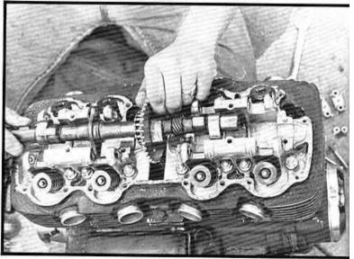
Before bolting down the valve head section it's advisable to pull the cam chain into place. With it in place proceed to tighten down the valve head retaining bolts. Next put the cam carriage units back into position followed by the cam. While sliding the cam into position place the chain so that it doesn't slip into crankcase. Mount the cam mounting block clamps and blocks then proceed to bolt the cam specket to cam shaft.
