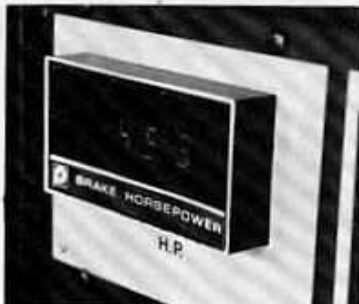
Patraco dyno reads horsepower directly. Engine rpm and load are held until reading stabilizes.
