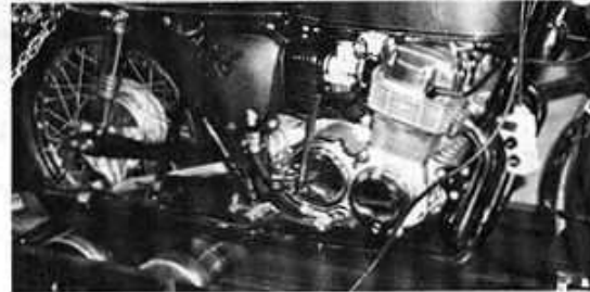
The Action Fours system is a four-into-two. It produced some fairly good readings, even without rejetting.
