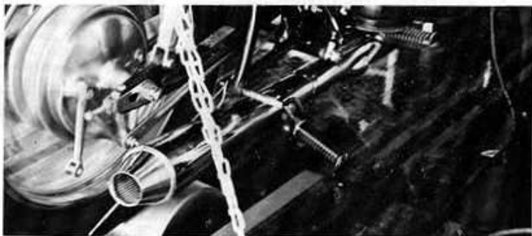
R. C. Engineering system ends in a big-bore muffler that passed plenty of gas and noise.
