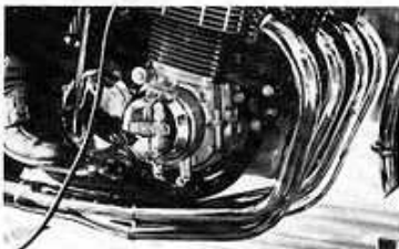
R.C. Enterprises' headers and collectors are welded into one piece. They look mean, but were not all that easy to bolt into place.
