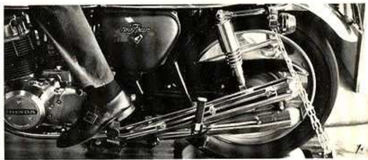
Patraco's engineers calibrated the dyno before the test was started. Readings on spring scale must match torque dial on panel.
