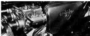
Single clamp holds R.C. setup to top frame tube. Design allows replacement of side covers, but not use of air cleaners.
