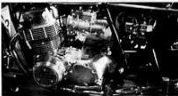
Wheel Specialties angled setup allows installation of air cleaners if desired, but prevents replacement of side covers.
