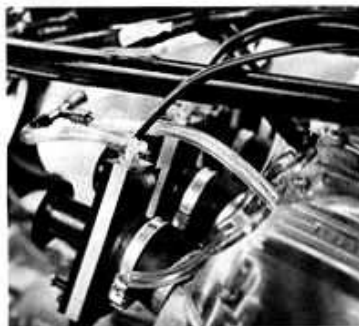
Extra-flexible fuel line has to be used with Lakes, since intake fittings move with slides.
