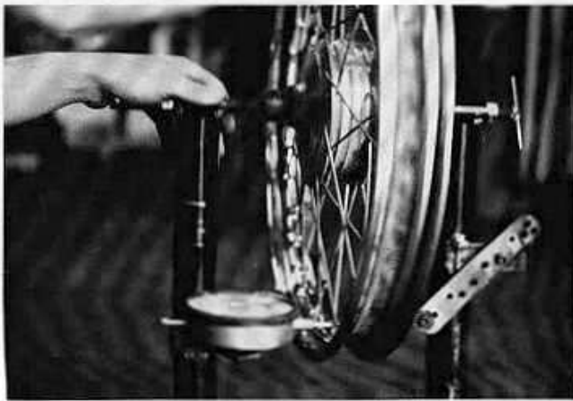
Arm mounted to the right glide leg is for checking horizontal run out.
