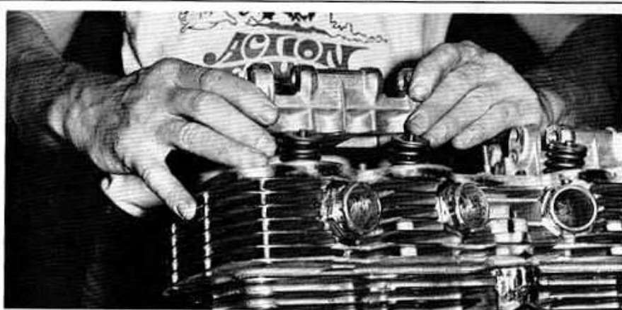
LEFT—Install the cam stands. Be sure that the four locating dowels are in position and blow the oil holes.
