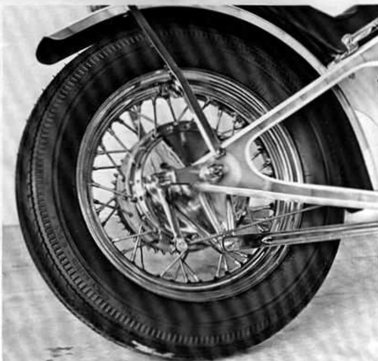
Fatter rear tire (5.10-16 Uniroyal shown) improves appearance, gives better ride and improved traction.
