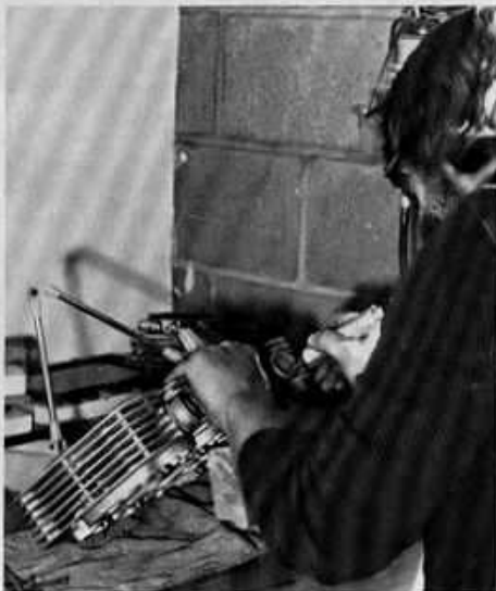
The two main heads used in the porting of a Honda head are shown above. These tools are a carbide cutter and a sanding head. The carbide cutter enables him to remove any burrs and rough casting left in the port. This is done through the intake port shown in photo at right.
