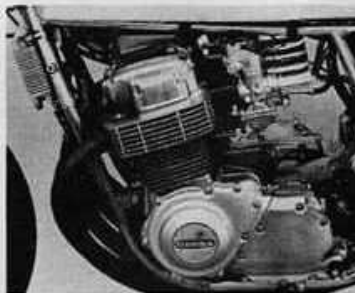
Competition engine mounts magneto in place of alternator, oversize Keihin racing carbs, scavenging exhaust system and high-volume oil cooler.
