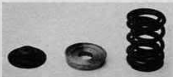
Competition springs and lightweight collars and retainers of the Yoshimura racing head provide valve sealing for the Daytona cam at engine speeds in excess of 10,000 rpm.
