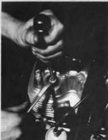
With feeler gauge between adjuster screw and valve stem, loosen lock nut and set tappet clearance.
