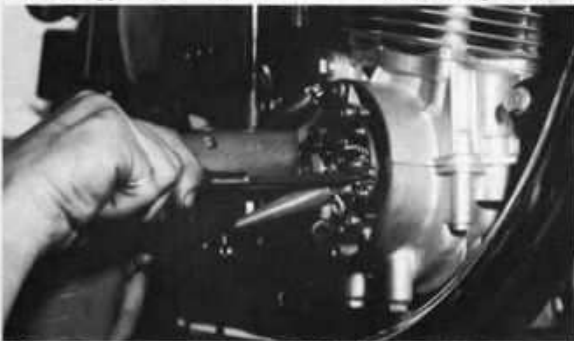
Adjust point gap at 21 degrees with dwell meter. After gap is set, set timing with a stroboscopic timing light.
