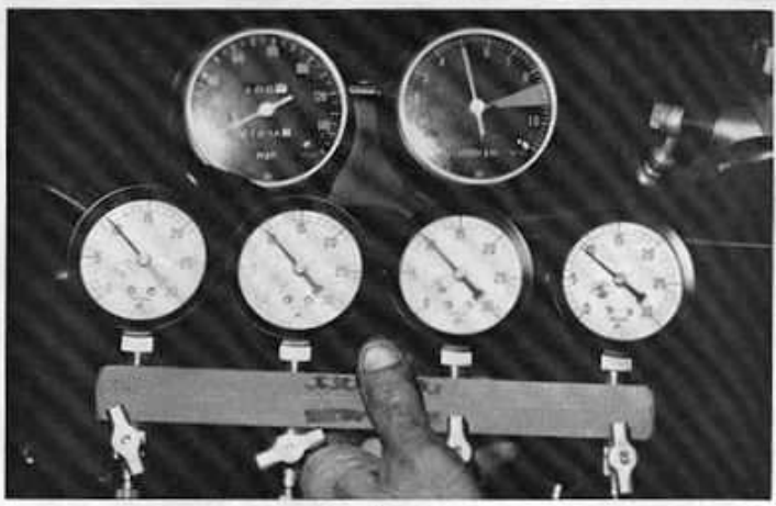
ABOVE —For cruising adjustment, all the needles should read near 10 inches.
