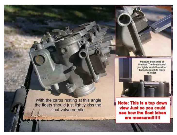
The carbs should set at an angle where the floats just barely rest against the spring loaded pins of the float valve needles but not leaning enough to where the weight of the float compresses the springs any but no so little that the floats do not keep the float valve needles seated. Above the floats are being set to 14.5mm for the PD series carbs measuring from the bowl gasket face.
