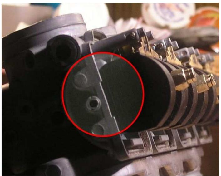
Here the notch you measure float level from is highligted. It is incorrect to measure from the gasket seat/face as some sources suggest or as how the PD series carbs are measured.
