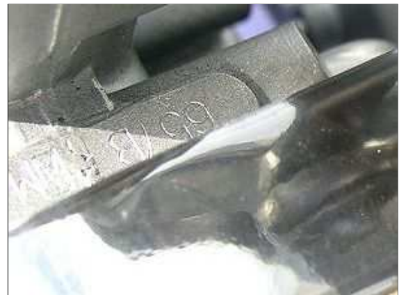
Casting numbers on the early style carbs is found on the top of the carb just behind the stay plate. It's stamped on a flat oval spot as shown above in the closeup.
