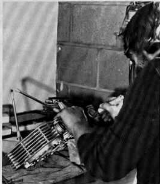
The two main heads used in the porting of a Honda head are shown above. These tools are a carbide cutter and a sanding head. The carbide cutter enables him to remove any burrs and rough casting left in the port. This is done through the intake port shown in photo at right.
