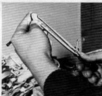
The port profile must be maintained for proper flow and performance. Here, the valve is being checked for size.
