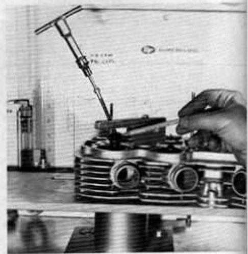
Flow bench operates by measuring amount of air that flows through port. Thus, intake valve has to be in place and depressed as if the engine were running.
