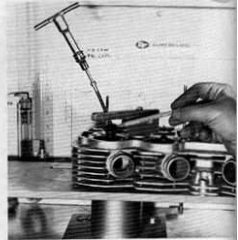
Flow bench operates by measuring amount of air that flows through port. Thus, intake valve has to be in place and depressed as if the engine were running.
