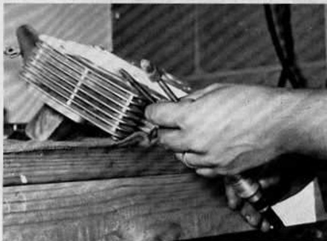
The two main heads used in the porting of a Honda head are shown above. These tools are a carbide cutter and a sanding head. The carbide cutter enables him to remove any burrs and rough casting left in the port. This is done through the intake port shown in photo at right.
