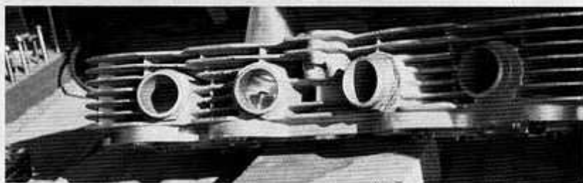
The #2 port on this Honda head was polished without porting. On the flow bench, the port actually flowed 2 cfm's less than a stocker!
