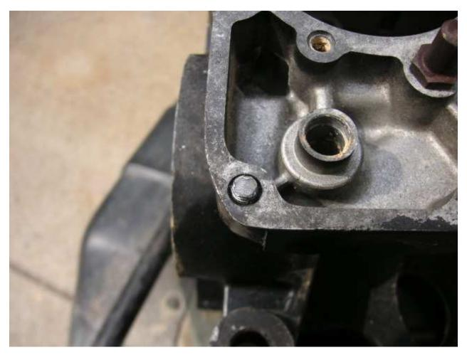
When a bolt is broken off, First thing is to take the cover off, if the nub of the bolt is still protruding out and theirs not enough to apply a wrench, Take a grinder and grind it down flush with the engine block. Make sure not to grind into the machined surface of the engine block.
