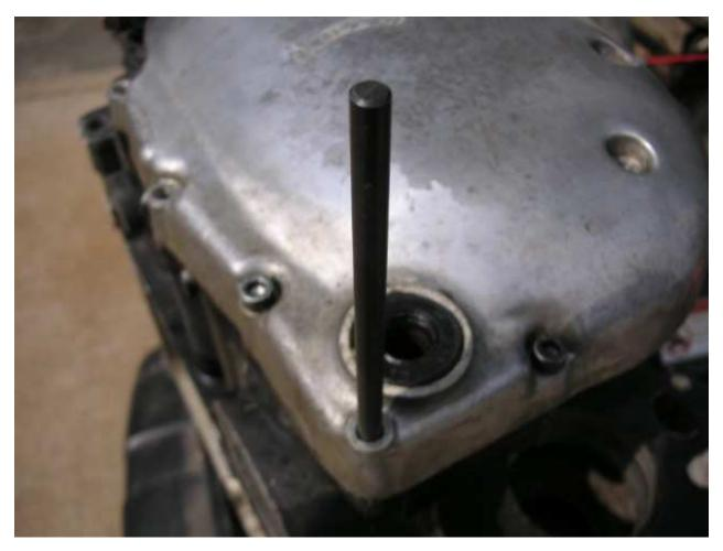
Once you have it flusheplace the cover and use only a couple bolts to hold it in place. Using a 1/4" center punch, Incert the punch into the hole that has the broken bolt and tap the punch until there's and indention in the center of the bolt.
