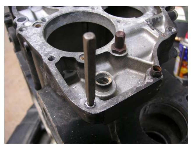
Using a 1/8" easyout, Tap the easyout down into the bolt until its tight. Take an ajustable wrench and screw it out. Do not get aggressive With an easyout, It will break
