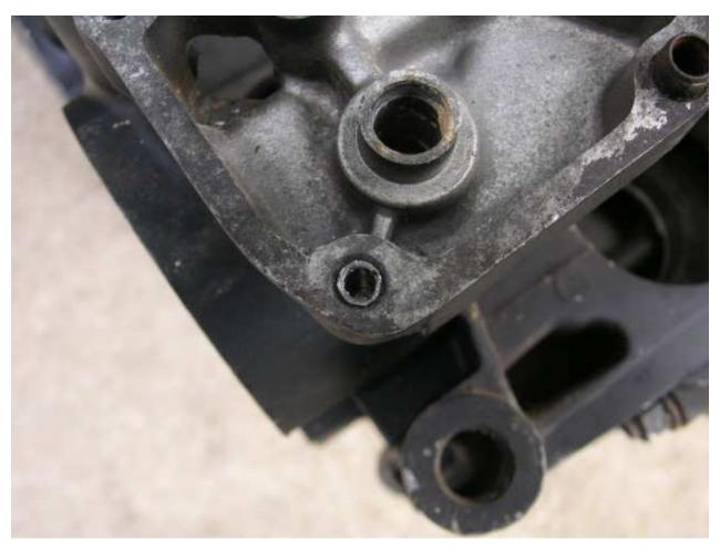
After drilling through the bolt, remove the drill bushing and cover. The hole in the center of the bolt will be the guide for the next size drill bits, Which is a 9/64" The last bit to use is a 5/32"before using an easy out, Fill the hole up with pentrating oil or PB blaster and let sit over night. This will better the chances of getting the bolt out.
