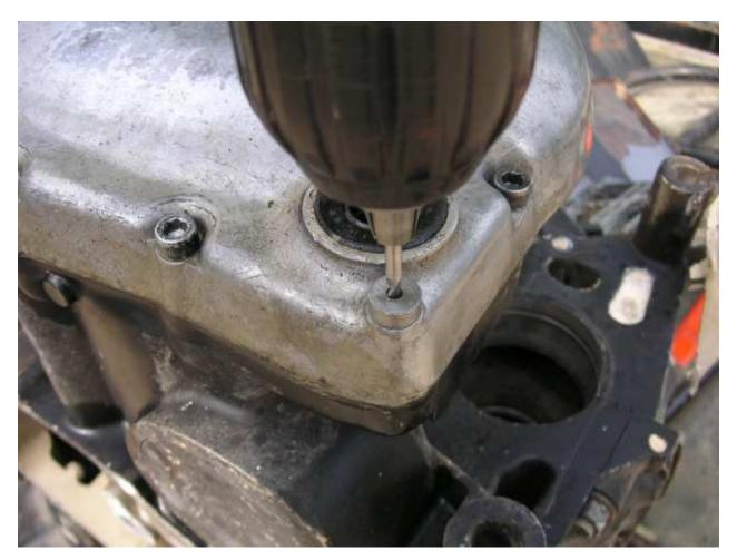
Place the drill bushing in the hole and with an 1/8" drill bit, start drilling. Do not apply alot of pressure as it will cause the bit to wonder. Take your time, when the drill bit gets close to the end of the bolt, it will in most cases start grabing more metal, Because the metal is getting thin at the end of the bolt and we don't won't to break the bit off in the bolt.
