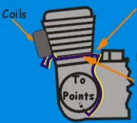
Re-route the blue wire and the yellow wire from the Ignition Points to the same color leads on the coils. Use the stock connectors.
