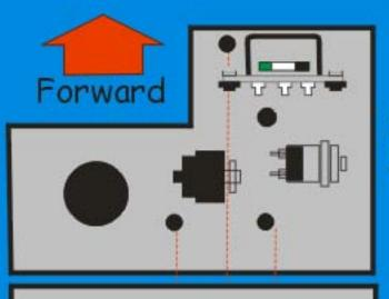
Attach assembly to box with 10mm nut & bolt - finger tight.
