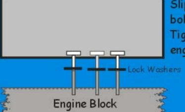
Slip three long 10mm bolts thru box. Tighten into the engine case. Recheck all bolts for tightness. Now reinstall the rectifier. Note that washer inside mount for extra spacing from the solenoid. Now install ignition switch, light switch and starter button. Don't tighten these in yet. You will probably want to remove them when wiring.
